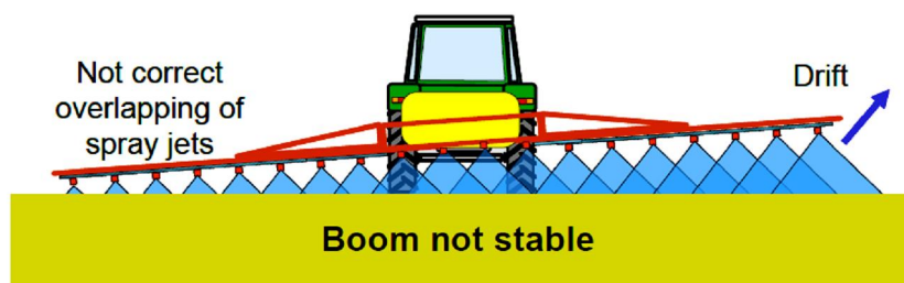
Figure 129: Consequences of an not stable boom sprayer.
